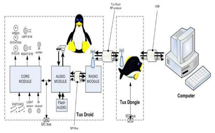
• The radio module includes an RF chip (ATR2406) and a processor (ATMEGA48). The RF chip is in charge of the physical layer. The radio processor manages the transport layer for streaming and control data. In order to provide full duplex audio with limited buffer sizes, the radio link is switching every 1 millisecond between emitting and receiving. The processor is also in charge of encapsulating / extracting the audio stream and controlling data in / from the RF frames.
