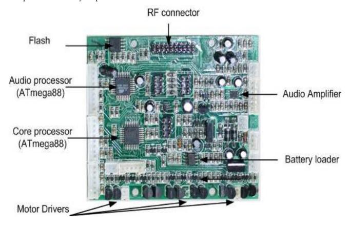
The link Mother Board Topology will provide you the detailed schematic of the main board.
