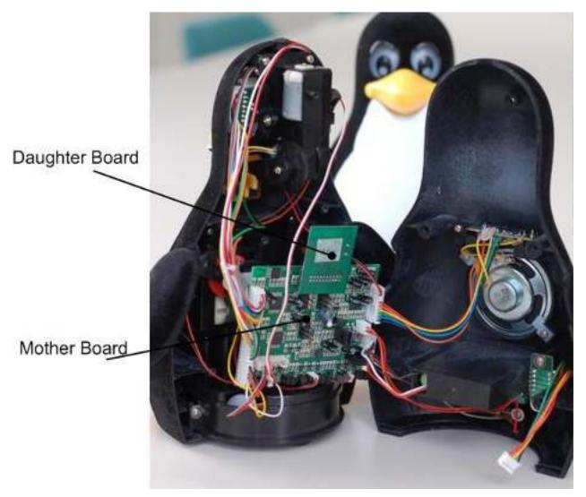
The daughter board is the radio part of Tux linking it to the dongle. The mother board is in charge of audio functionalities, sensors and actuators control plus battery charging.
